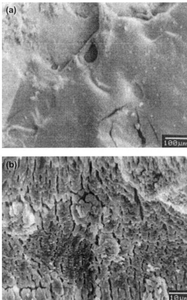
**Figure 4.** SEM photographs of (a) raw bone and (b) bone heated at 500°C.
