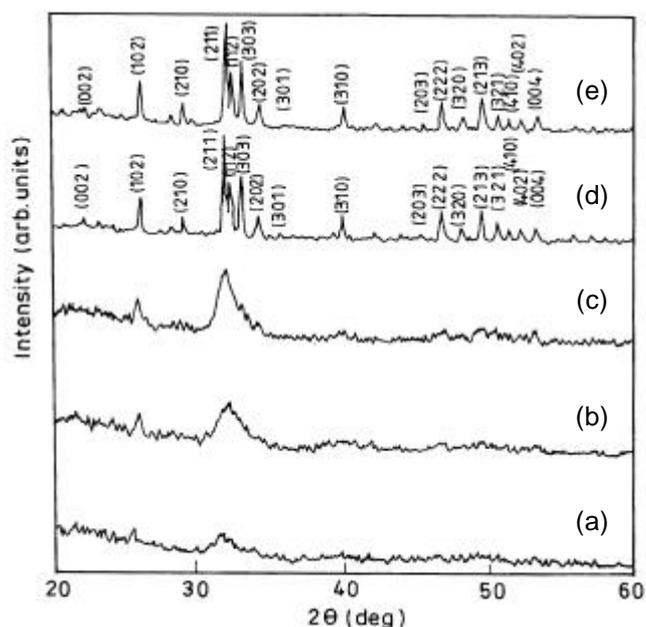
**Figure 2.** XRD patterns of (a) raw bone and bone heated at (b) 300°C, (c) 500°C, (d) 700°C and (e) 900°C.
